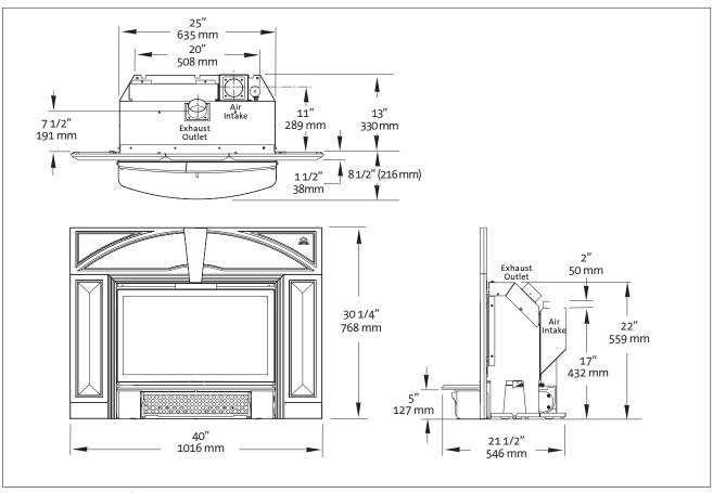
Figure 1. GI 425 DV dimensions.
